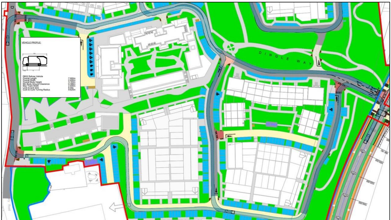
Figure 5-18 - Refuse Vehicle Track through the development
